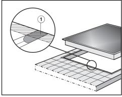
The grouting ① and the shaded area under the frame of the ProLine element must be smooth and flat so that the frame will sit evenly on the countertop and so that the sealing strip under the top edge of the ProLine element can provide an adequate seal with the countertop.
